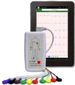
The **EC-12RM** is a compact ECG device, which can forward real-time, 12-channel ECG signals to any Android and iOS device (e.g.: tablet or smartphone) via Bluetooth or Wifi connection. This way the device can make excellent quality ECG records in a mobile and fast method. We can measure certain sections of the ECG and customize the on-screen display of the ECG to suit our own needs.
