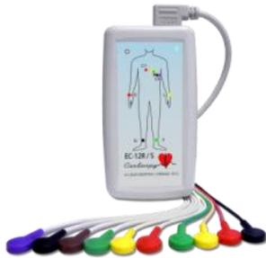
**EC-12R/S** ECG has all the characteristics of the EC-12R device but it can also be used for making stress test examinations without monitoring blood pressure. Connected to a PC, the device offers high precision sampling, good quality ECG curves with the aid of mains, muscle and baseline filters. The analysing SW performs continuous HR, ST, BP trends, MET and rhythm analysis.
