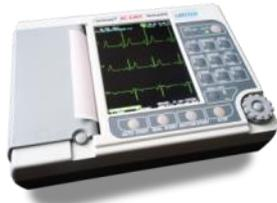
The **EC-12RT** is a high-profile portable ECG machine with thermal printer and coloured TFT monitor. The small, lightweight and compact device is very user-friendly, its TFT display, alphanumeric keyboard and various extra functions make it easy to use. Its sophisticated filters and amplifiers ensure a top-quality ECG recording.
